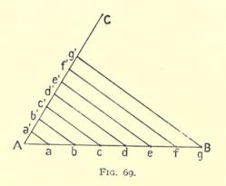
Since the triangle aAa' is a right-angled triangle, having its right angle at a', the scale of longitude can be found as follows:
