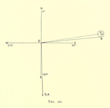
to be  $195^{\circ} 23'$ , it follows that the magnetic north must lie either  $195^{\circ} 23'$  to the left of A, or  $360^{\circ} 00' - 195^{\circ} 23'$ , i.e.  $164^{\circ} 37'$  to the right of A as shown in the following sketch.
