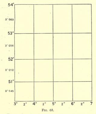
Draw in the lower horizontal line, and mark it off in equal spaces of two inches each to the limits of the longitude required.
