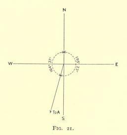
Now set the vernier either  $195^{\circ} 23'$  to the left of A or  $164^{\circ} 37'$  to the right of A. The sight wire will now be pointing direct to the magnetic north.
