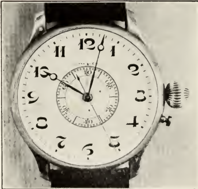
FIG. 209.—Standard second-setting navigation watch.
