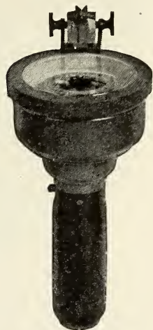
FIG. 36b.—0.6 aperiodic observer's compass.
