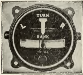
FIG. 100.—Combined turn-and-bank indicator.
