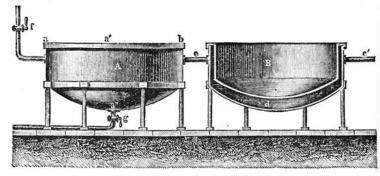
Fig. 32.—Steam-heated kettles.
