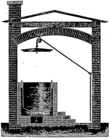
Fig. 30.—Free-fired pan for boiling oil.
