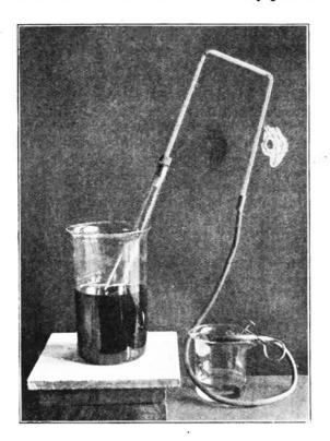
Fig. 27.—Trimble's apparatus for tannin determination.
