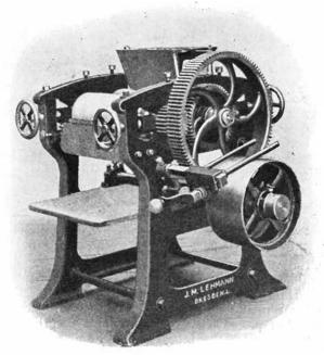
Fig. 38.-Lehmann's Grinding Mill.
