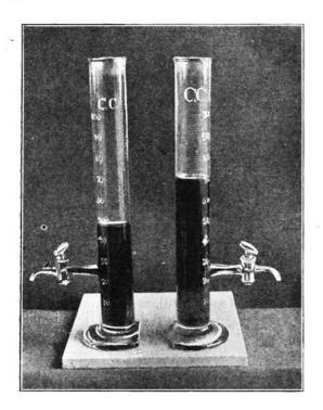
Fig. 28.—Hehner's Nesslerising tubes.
