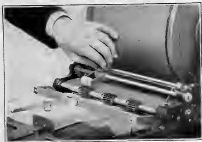
Adjusting Idler Feed-Roller for narrow sheets
