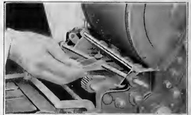
Removing Idler Feed-Roller and Shaft
