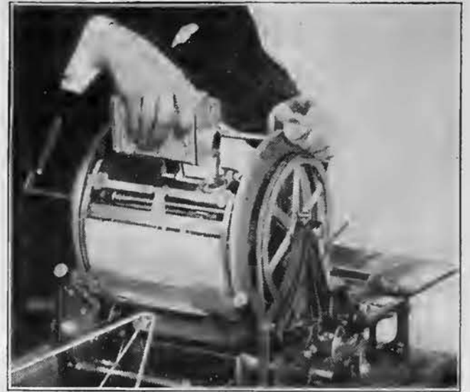
Proper method of filling the Ink Fountain
