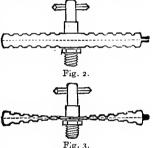
held from the plate by  $F_{ig. 3}$ . the finely pointed screws, "C," "C," these screws also being used to finely regulate the tension upon the chamber, "A." The knife edge, "E," is inserted in the post of the vacuum chamber (which passes through a hole in the spring, "D,") thus pulling the two corrugated discs of the vacuum chamber apart, leaving it in a poise with the atmosphere.
