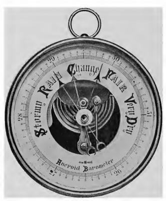
Aneroid Barometer with C. & T. Patent Altitude Adjustment
