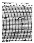
one advantage of the barograph. Two observations of an aneroid were made (at 10 p. m. and 8 a. m., respectively) both showing a reading of 30.10 in., which would indicate a "stationary" barometer with a continuance of present weather. A glance at the barograph record shows a rapid fall and rise between 10 p. m. and 8 a. m., which indicates a short but severe storm due at about 11 a. m.
