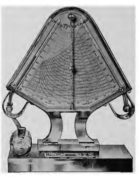
The Hygrodeik is an improved form of hygrometer, being portable, easy to read and very accurate.
