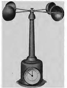
Fig. 1. Robinson's Anemometer
