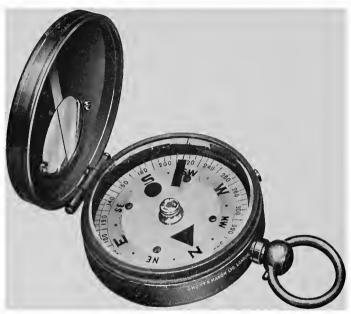
Fig. 6. Luminous Dial Compass.
