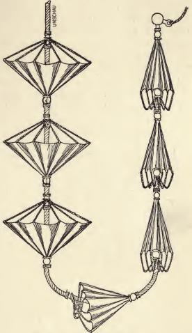
FIG. 129.—Water anchor for balloon. (From "Die Umschau.")
