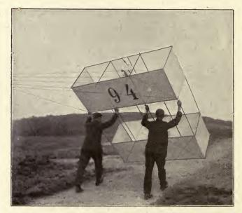
FIG. 161.—Ascent of a box-kite containing meteorological instruments (Photograph by the Berliner Illustrationsgesellschaft.)
