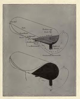
Fig. 116.—Drawing showing the design of the kite-balloon.
