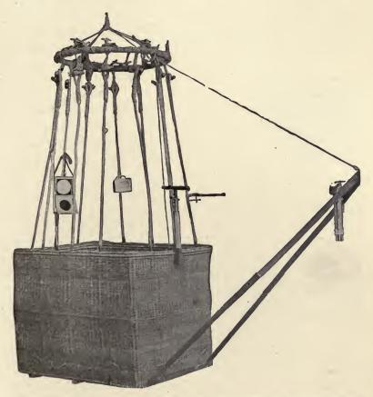
FIG. 150.—Basket fitted with instruments according to the method proposed by Assmann.
