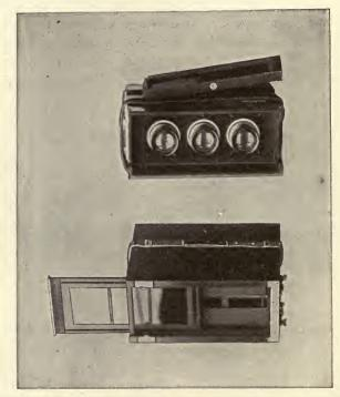
FIG. 213.—Miethe's camera for three-colour photography in a balloon. At the top is shown the front part with the three lenses, and below is seen the sliding screen carrier and the shutter.
