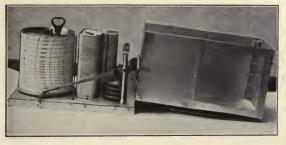
FIG. 119.—Barograph, or recording barometer.
