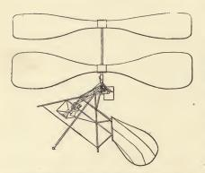
FIG. 49.—Dufaux' flying machine with propellers.
