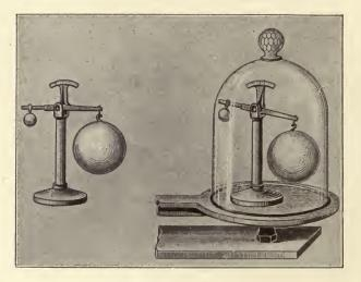
FIG. 14.-The Baroscope.
