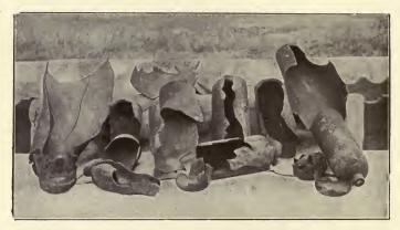
FIG. 100.—A collection of exploded gas cylinders.
