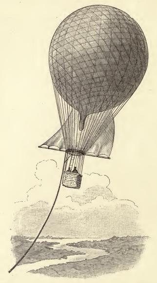
FIG. 19.—Balloon with sail, and with guide-rope fastened to the ring.
