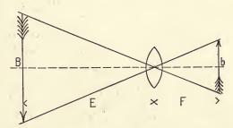
FIG. 197.—Diagram showing the relation between the focal length of the lens, the size of the image, and the distance of the object.
