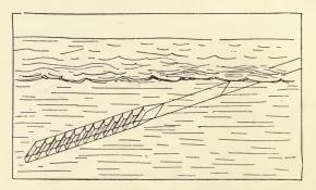
FIG. 134.—Deviator offering the maximum resistance. (From "Die Umschau.")
