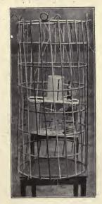
FIG. 158.—A wickerwork basket with instruments for a recording balloon.
