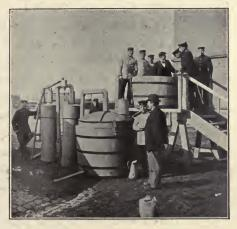
FIG. 147.—Apparatus for generating hydrogen.
