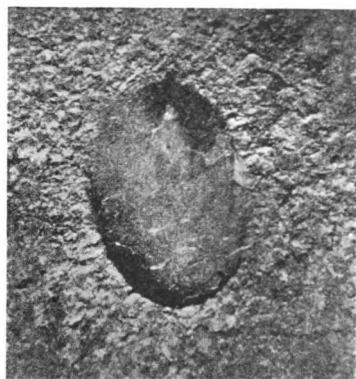
FIG. 24.—Photomicrograph of fused focus-spot in a tantalum anticathode.
