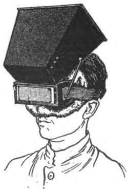
FIG. 2. Dessane's fluoroscope elevated to the top of the head after the fluoroscopic examination has been made, permitting the operator to see by ordinary light without losing the sensibility of the retina because of a ruby glass which automatically drops in front of the eyes as the fluoroscope is elevated.
