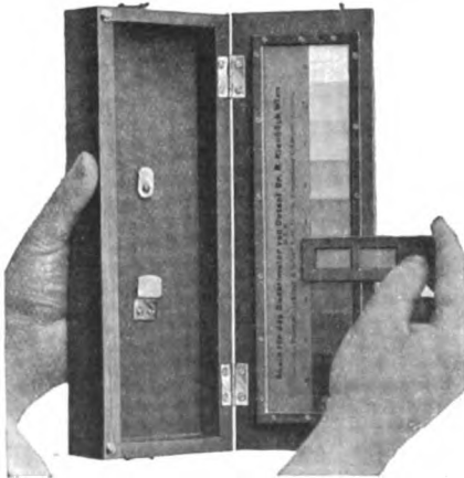
FIG. 344.—Comparing the wet strip with the standard scale, using the slide.
