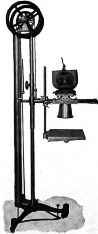
Fig. 61. A pedestal, with a lead glass protection shield, compression cone and plate holder.
