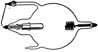
FIG. 13.-Valve tube.
