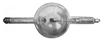
FIG. 11.-The Coolidge tube.
