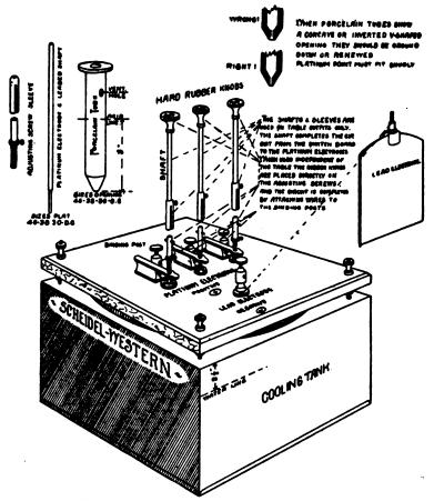
FIG. 14.—The Wehnelt electrolytic interrupter.
