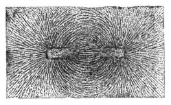
FIG. 4.-Action of bar magnet on iron filings.
