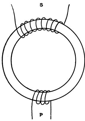
FIG. 16.-Ring type of transformer.
