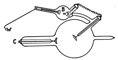
FIG. 10.--Queen's self-regulating tube.
