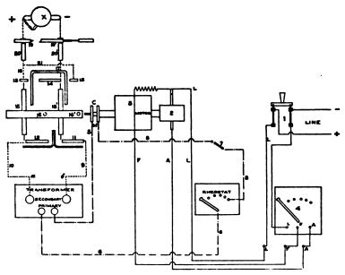
FIG. 17.-Diagram of connections of interrupterless apparatus.
