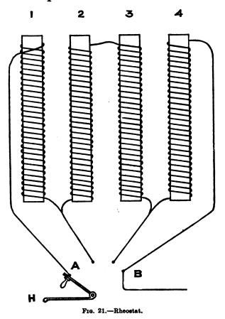
the current flows directly from H through the movable arm to B, the rheostat no longer being in the circuit.
