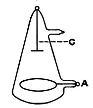
FIG. 7.-Early type of Röntgen-ray tube.
