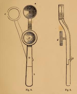
two handles can be separated or allowed to come close to each other. By this means an exact focal distance can be obtained. A drop of fluid con-
