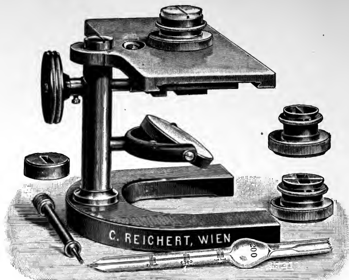
FIG. 11.—FLEISCHL-MIESCHER HEMOGLOBINOMETER. (Wood.)
