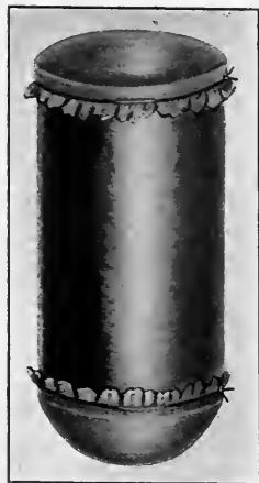
FIG. 7.—A Vertical Cylinder closed at either End by an Elastic Diaphragm and Filled with Fluid.
