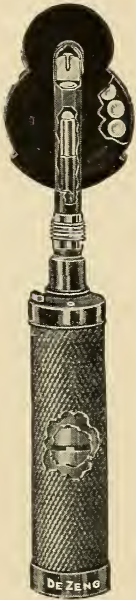
FIG. 13.—A simple electric ophthalmoscope (one-half the actual size) for the determination of the presence or not of an increased intracranial pressure, and its degree, by the direct method. Two small electric batteries are enclosed in the cylindrical metallic handle so that this useful instrument may be easily carried in a coat pocket—its weight being less than one-half pound. Its simplicity and durability minimize the necessity of repairs from careless handling. The very early stages of papilledema, as well as the advanced degrees of “choked disks” can be accurately measured without the necessity of artificial light or the interposition of lenses, as required by the former indirect method of ophthalmoscopic examinations.
