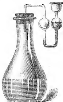
FIG. 109.—Flask for the Approximate Estimation of Sugar by Fermentation.
