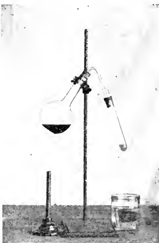
Fig. 32.—A simple distilling apparatus.
