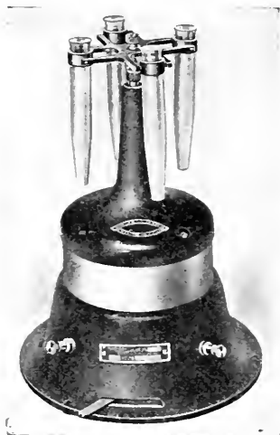
Fig. 20.—The Purdy electric centrifuge with four arms.
