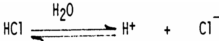
Figure 3-2. The ionization of hydrochloric acid.
