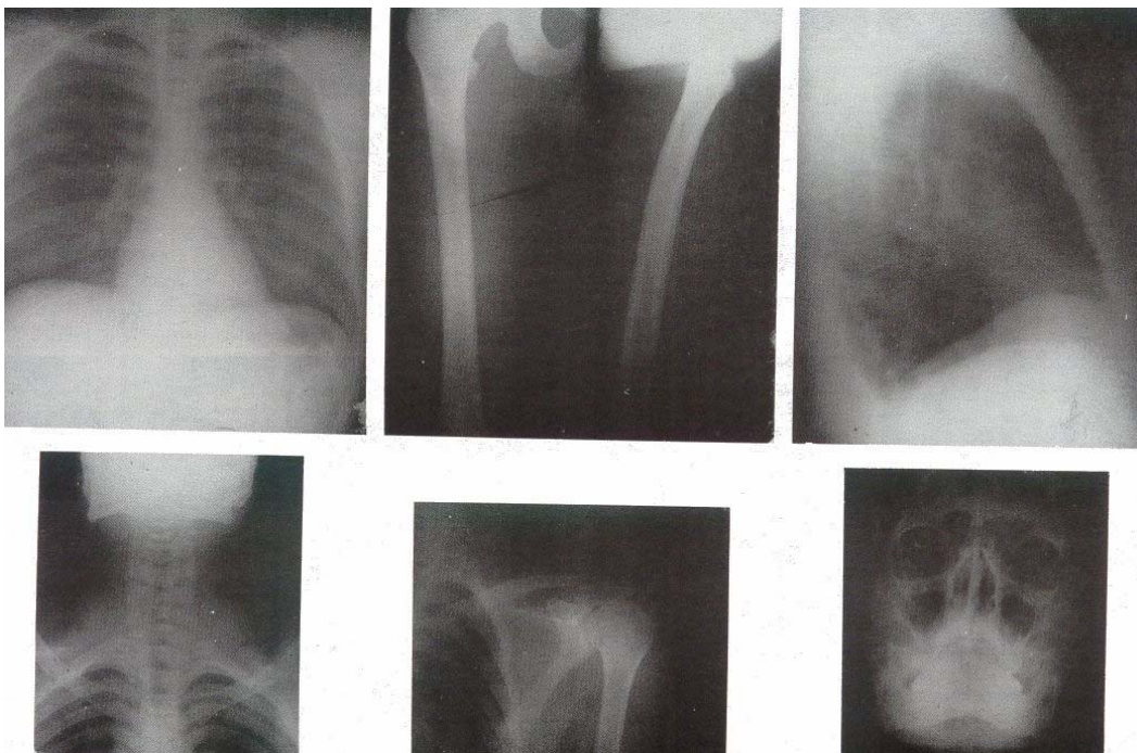
Figure 1-12. Radiographs that exhibit evidence of SR fog. Note similarity of image appearance and general loss in satisfactory contrast.
