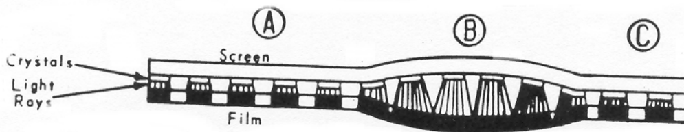
Figure 2-11. Poor screen contact produces a blurred radiographic image. In areas A and C the film and screen are in good contact. In area B, light rays from one crystal cross those of others, and the resultant image of each crystal blurs into those of the adjacent crystals.
