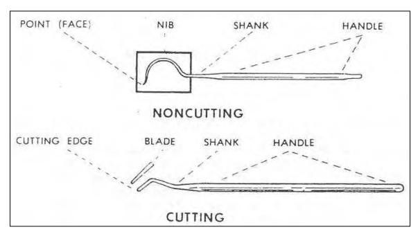
Figure 1-1. Parts of a hand instrument.
