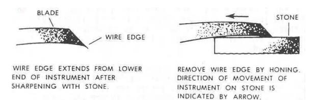
NOTE: Using a hand stone, the instrument should be stabilized while being sharpened. the instrument is placed so the inner concave surface is upward and parallel to the floor. The stone is placed on the inner surface of the blade at its junction with the shank and then moved back and forth in a sawing motion until it reaches the tip. The outer surface is honed slightly to remove the wire edge.
