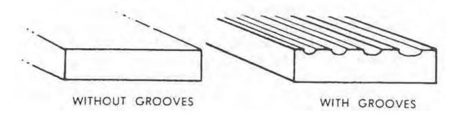
Figure 1-2. Flat sharpening stones.
