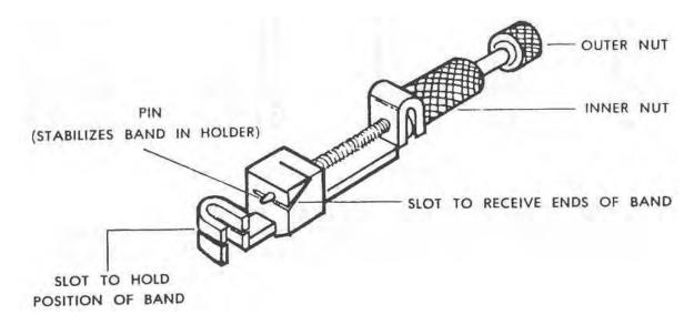
Figure 2-10. Tofflemire matrix retainer.
