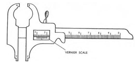
Figure 5-5. Millimeter (Boley) gauge.
