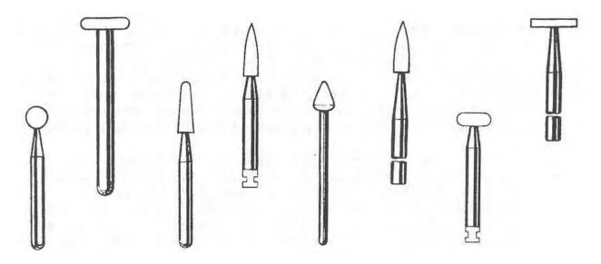
Figure 2-27. Mounted abrasive stones and wheels.
