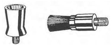
Figure 2-28. Polishing cup and polishing brush.
