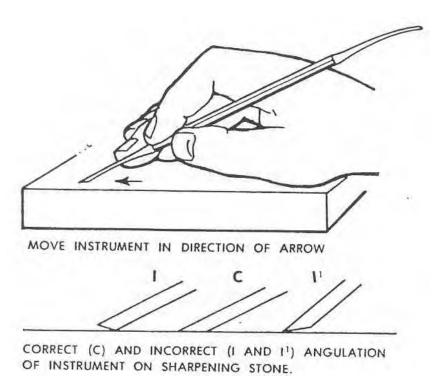
Figure 1-3. Proper angulation for sharpening an instrument.
