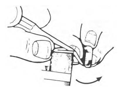
Figure 1-5. Sharpening an instrument using a hand stone.
