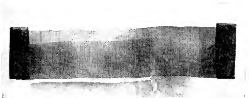
FIG. 73.—Wire gauze roll; size, 100 to the inch.
