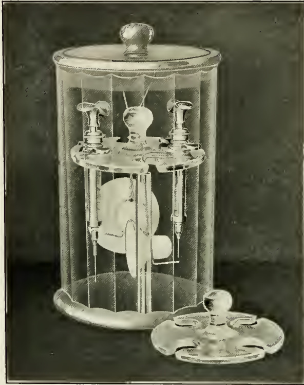
FIGURE 30 Glass jar with ground cover and glass tray to hold syringes and cups.
