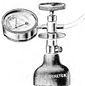
FIG. 26. -Coxeter's pressure gauge for oxygen cylinders.
