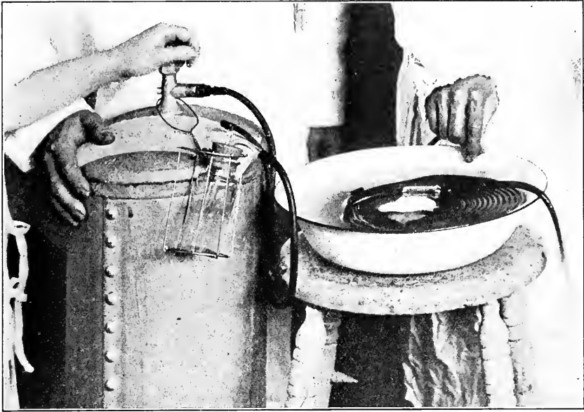
FIG. 14.—OXYGEN PASSING THROUGH RUBBER COIL IMMERSSED IN HOT WATER (Service of Dr. Bainbridge).
