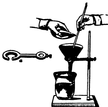
Pouring with a guiding rod.
