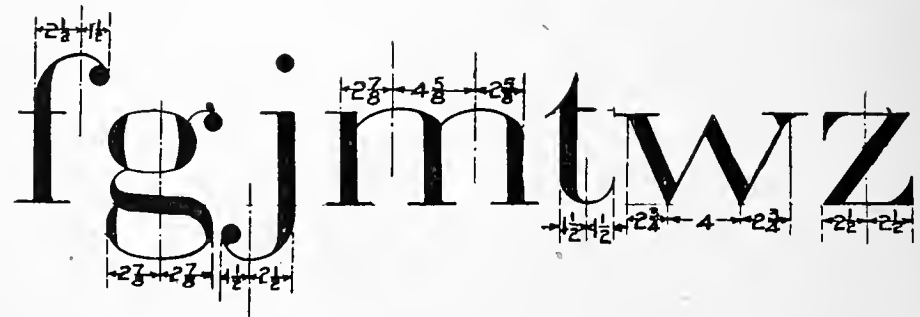
Fig. 76.—Modified Center Line Spacing Guides for the Roman Small Letters Shown.
