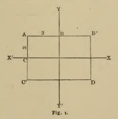
distances apart may be easily obtained if their distances from two intersecting straight lines are known. For instance, the position of the point A is accurately de-
