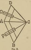
since AD = AB + BE, find DE, distance traversed by the piston while the crank moves through any given angle.
