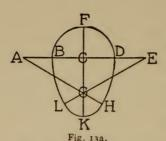
26. How many square feet in the section of a sewer (see figure) whose dimensions are as follows:
