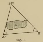
tance from a point A to an inaccessible object P; further, imagine a wood W so situated that B would be the first point to the right of A from which an unobstructed view of P could be obtained. Now, we might lay off a known length AB (called a base line) and with a transit, measure the angles BAP and ABP; we could then calculate the
