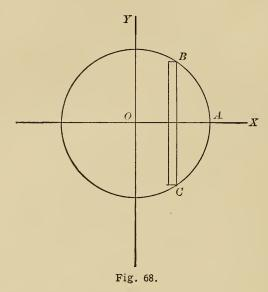
255. Moment of inertia of an ellipse about its minor-axis.
