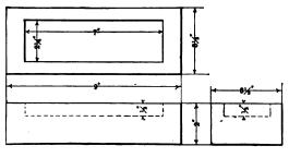
is to be 7 in. long, 2 $\frac{1}{2}$  in. wide, and  $\frac{1}{2}$  in. deep. This cut represents a working drawing such as is given to the carpenter. Find the number of square feet of lumber required to make the blocks, allowing as
