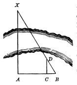
5. To find the distance from A to the inaccessible point X: Draw AB perpendicular to AX. Join BX. Draw CD parallel to AX. What kind of angles at A and C? What two similar triangles? What sides are measured? What is the proportion? Show how you can find the distance from B to X.
