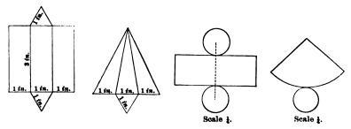
prism and a triangular pyramid of the same base and altitude, and a cylinder and a cone of the same base and altitude. Fill each with dry sand, and find, by measuring or weighing, the relative size of the prism and pyramid and of the cylinder and cone. Since this ratio is true between all kinds of pyramids and their corresponding prisms, and between all cylinders and cones whose bases and altitudes are equal, what general rules can you give for finding the volume of pyramids and cones ?
