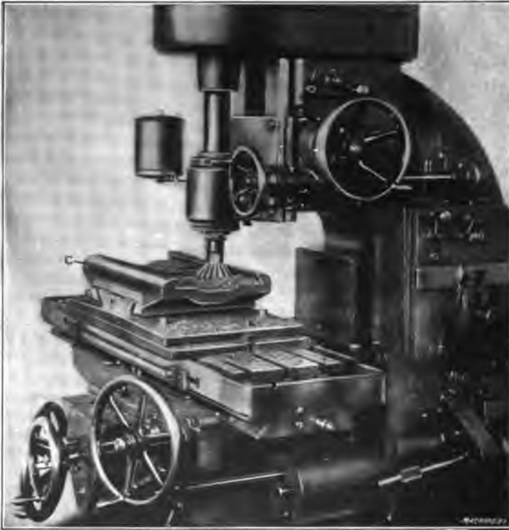
Fig. 20. Example of Milling on Vertical Milling Machine
