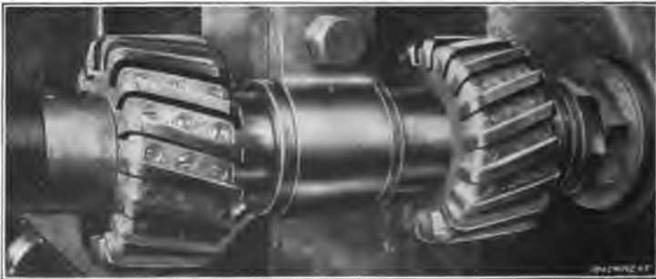
Fig. 33. Cutters used for Channeling Main-rod
