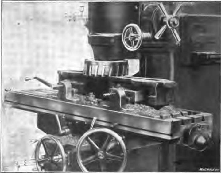
Fig. 26. Machine equipped with Two Work-holding Fixtures so that One Casting can be chucked while the Other is being Milled
