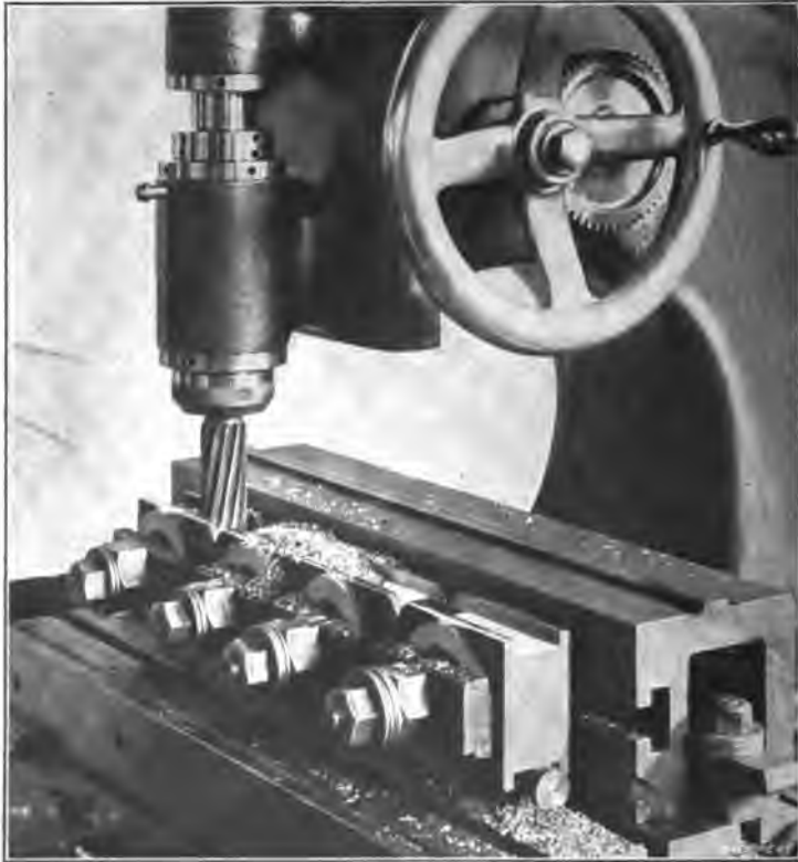
Fig. 22. Milling Connecting-rod Bearing Brasses on Becker Vertical Machine
