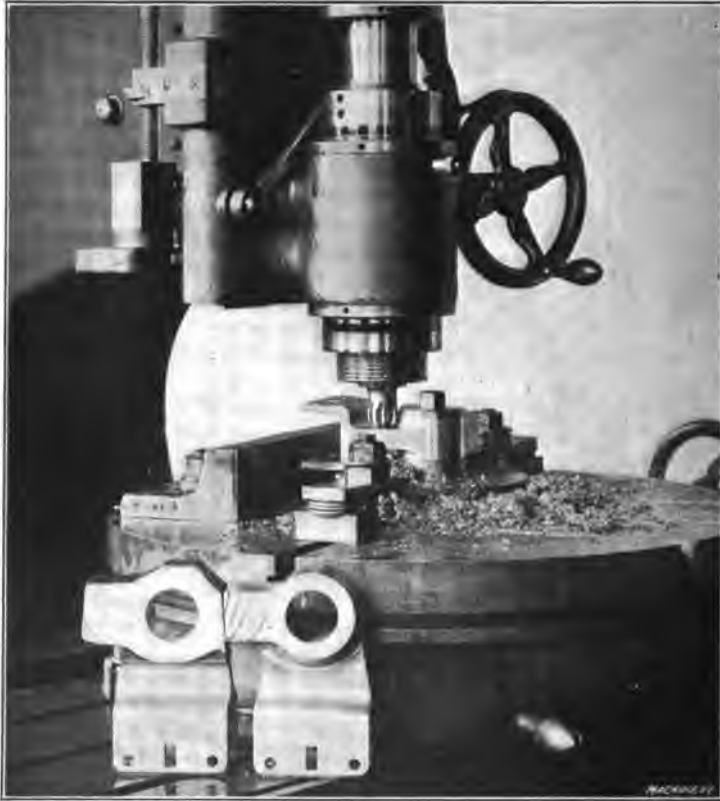
Fig. 24. Finishing a Circular Fillet with a Rose Milling Cutter
