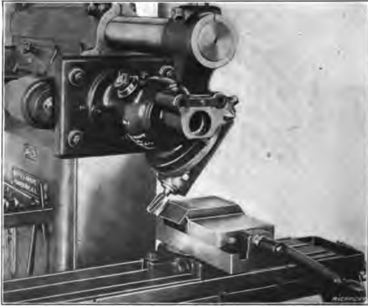
Fig. 38. Vertical Attachment applied to a Horizontal Milling Machine
