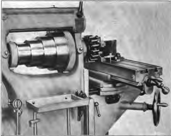
Fig. 27. Finishing Vertical Surface with Face Mill
