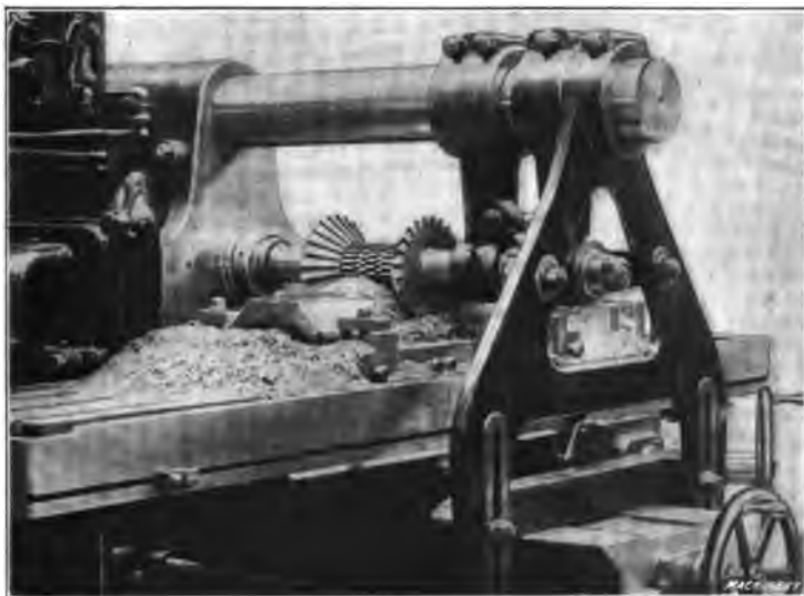
Fig. 23. Another Gang Milling Operation
