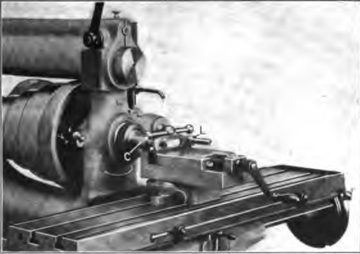
Fig. 25. Milling Slot with End Mill
