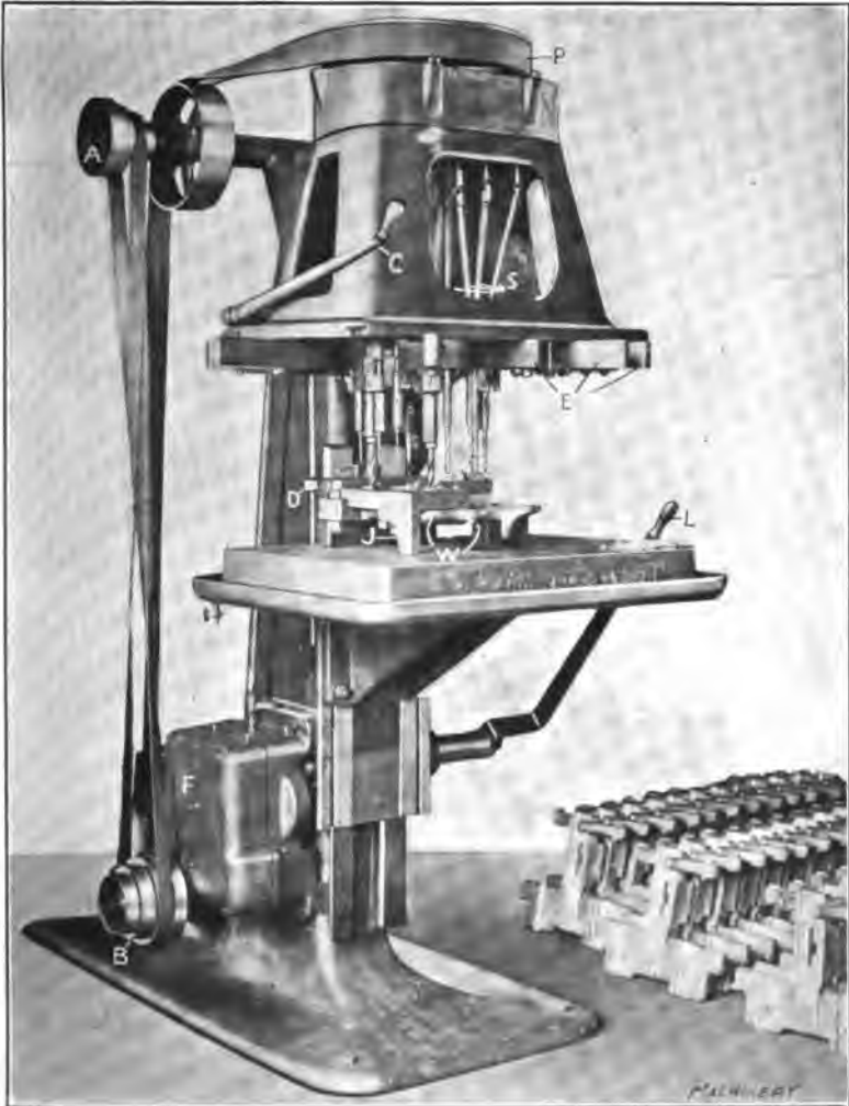
Fig. 81. Pratt & Whitney Adjustable Multiple-spindle Drilling Machine
