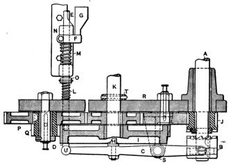
Fig. 7. Turret Lathe Indexing Mechanism to be assembled
