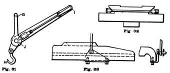
Fig. S1. Crane Attachment, for ascertaining whether a Piece being lifted from its Seat binds. Fig. S2. Device for lifting a Swivel by Hand. Fig. S3. Method of attaching a Lifting Device to a Turret Carriage
