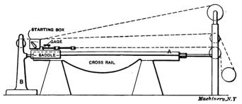
Fig. 25. Pulling Machine, Fig. 22, and Tension Indicator, Fig. 23, in Position for Moving a Planer Saddle along the Cross-rail
