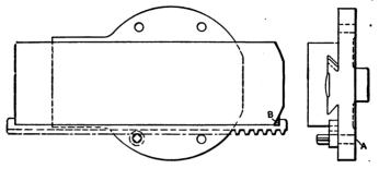
Fig. 16. Device for Pulling Planer Slide Back and Forth
