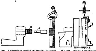
Fig. 35. Appliances which Facilitate placing the Face-plate on the Lathe Spindle
