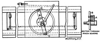
Fig. 20. Rack and Pinion for Pulling a Planer Saddle
