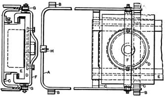
Fig. 38. Device used when fitting a Saddle to a Cross-rail
