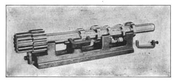
Fig. 2. Jig for Drilling Pin-hol≏s in Collars on their Shaft to Insure Interchangeability
