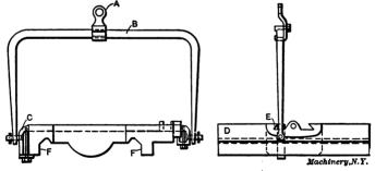
Fig. 30. Sling for Lifting Lathe Carriages, which is equipped with an Adjustable Crane-hook Eye
