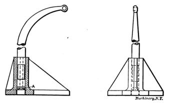
Fig. 37. Small Individual Crane provided with Ball Thrust Bearing
