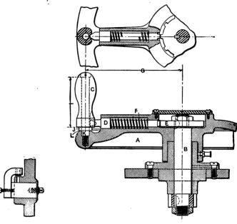
Fig. 12. Jig for Setscrew Holes
