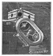
Fig. 8. Assembled Turret Lathe Indexing Mechanism shown in Detail in Fig. 7
