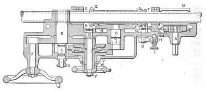
Fig. 9. Engine Lathe Apron to be assembled
