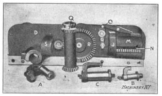
Fig. 11. Testing Fixture for Parts of Lathe Apron
