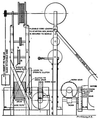
Fig. 22. Pulling Device for Large Planer Saddles
