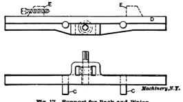
Fig. 17. Support for Rack and Pinion
