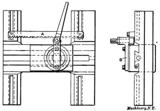
Fig. 19. Method of Attaching Rack and Pinion to a Lathe Rest
