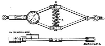
Fig. 23. Indicating Mechanism for Pulling Device
