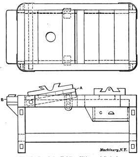
Fig. 18. Bench for Holding Slides and Swivels
