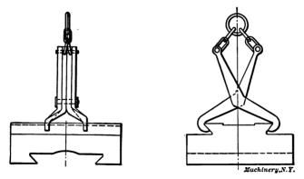
Fig. 34. Gravity Tongs for Handling Work such as illustrated
