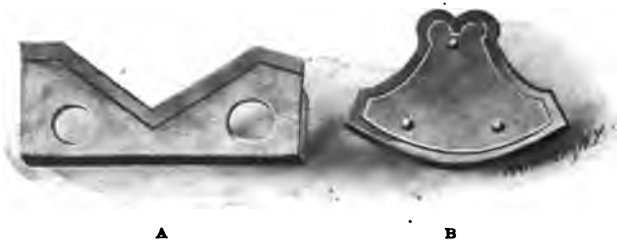
Fig. 11. Drop Hammer Die and Punch with Shields
