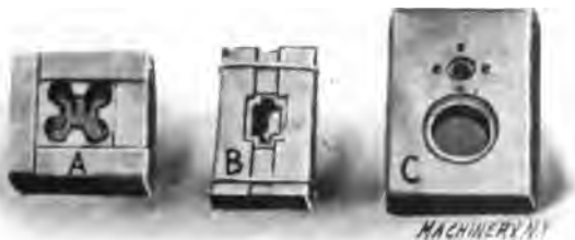
Fig. 10. Square Threading Die and Press Dies with Covers in Place, Ready for Hardening
