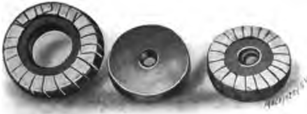
Fig. 12. Two Drawing Dies Prepared for Local Hardening and One Without Cover
