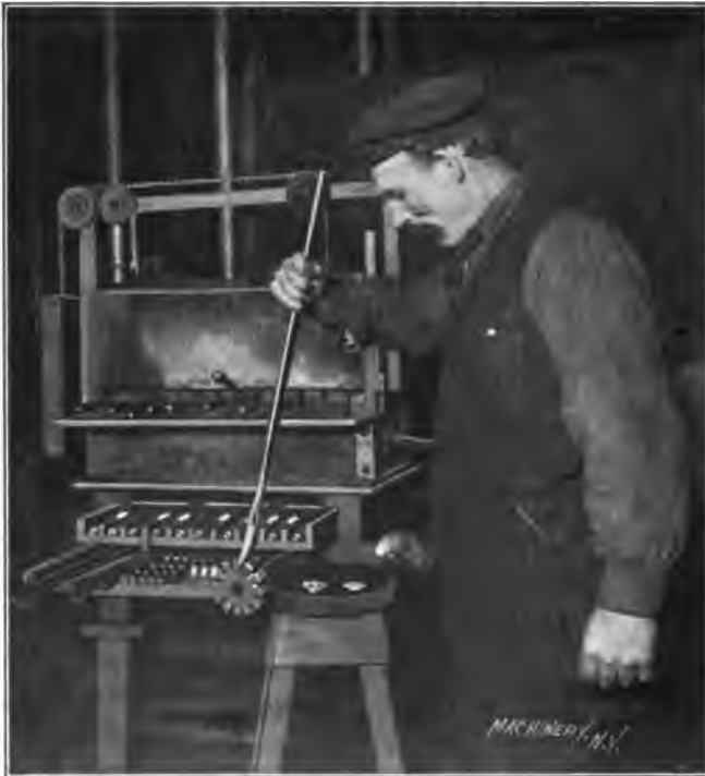
Fig. 22. Testing a Milling Cutter, when Hardening, by Swinging it Back and Forth past a Magnetic Needle
