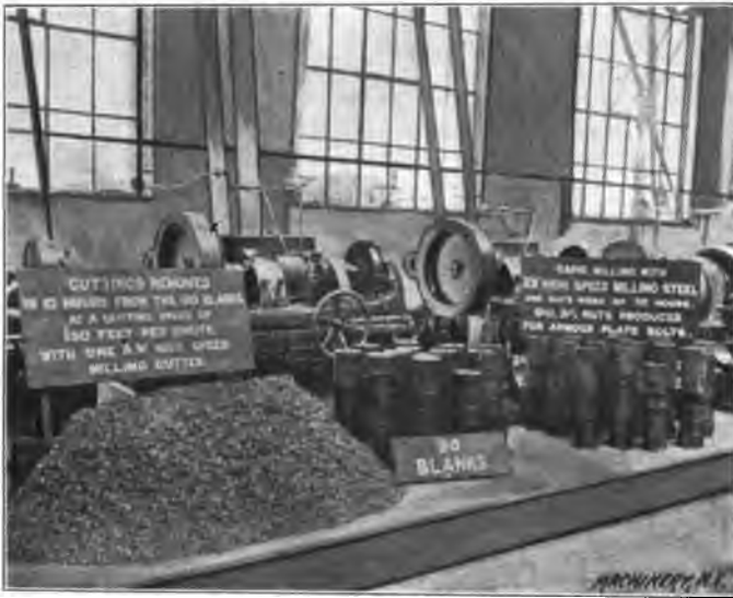
Fig. 9. Making Hexagon Nuts from Rolled Bars with Cutters made from High-Speed Steel. Ninety Nuts Produced in a Day of Ten Hours.
