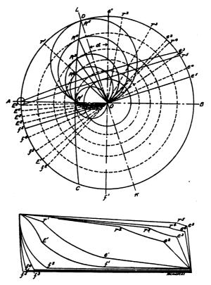
Fig. 9. Zouner's Diagram, Illustrating the Change of Valve Events for Different Points of Cut-off
