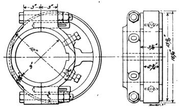
Fig. 18. Eccentric for Consolidation and Atlantic Type Locomotives
