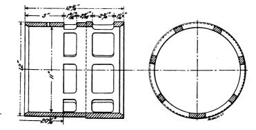
Fig. 11. Valve Chest Bushing for Atlantic Type Locomotive
