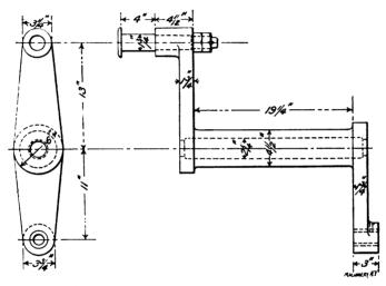
Fig. 17. Indirect Rocker Arm for Consolidation Locomotive
