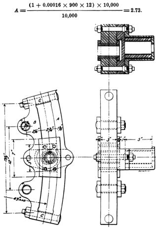
Fig 21. Wrought Iron Oase-hardened Link for Consolidation Locomotive
