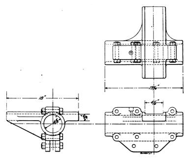
Fig. 25. Rocker-box for Consolidation Locomotive
