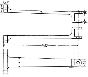
Fig. 20. Eccentric-rod for Consolidation Type Locomotive
