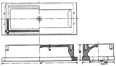
Fig. 15. Balanced D-valve for Consolidation Locomotive
