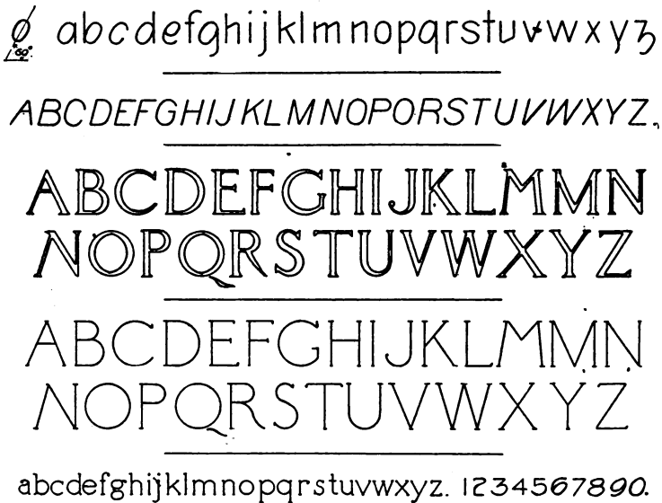
Fig. 28. Alphabets for Lettering on Drawings
