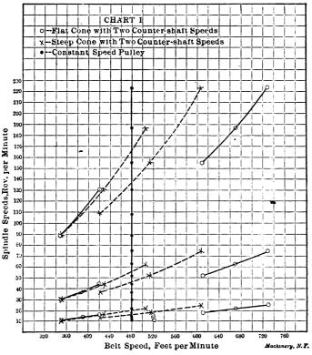
Fig. 3. Variation in Belt Speeds for Various Methods of Driving.
