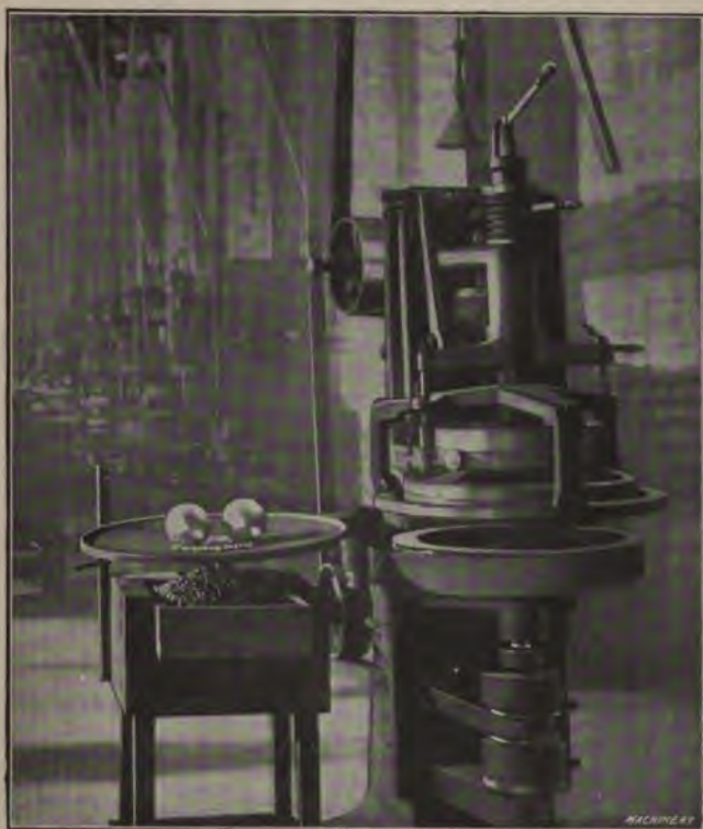
Fig. 32. General View of the Grant Dry Grinding Machine, with Samples of Largest and Smallest Balls ground in it
