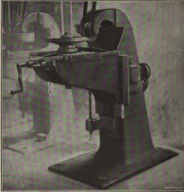
Fig. 33. Special Grinding Machine used for Grinding the Segments for the Path of the Balls in the Machine shown in Fig. 32
