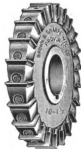
Side-milling Cutter with Inserted Teeth FIG. 567.
