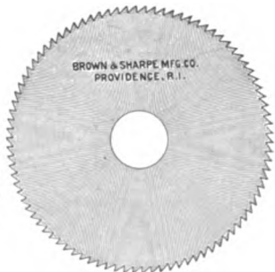
Screw-slotting Cutter. FIG. 570.
