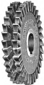
Interlocking Side-milling Cutter. FIG. 559.
