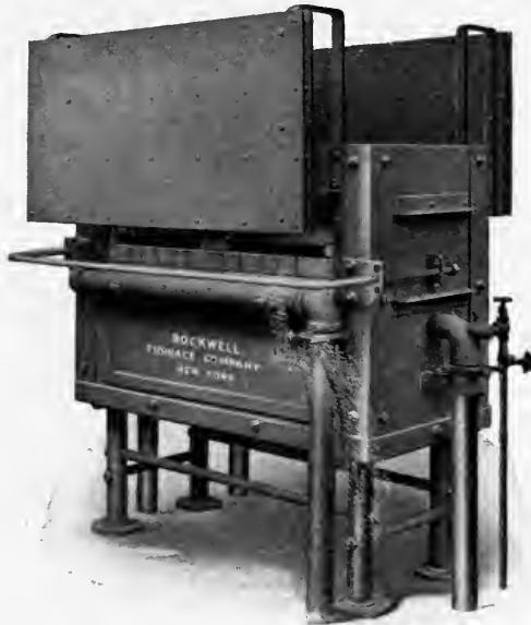
FIG. 157.—Double opening forge for center heating.
