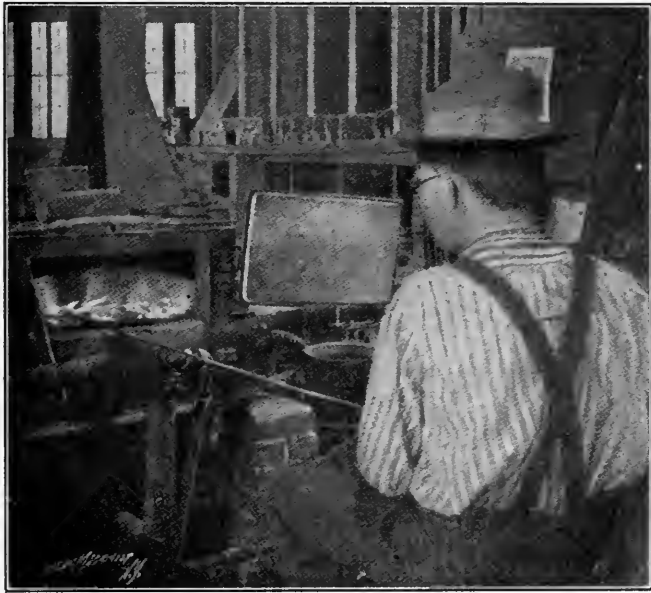
FIG. 205.—Heating flanges in muffle, using natural gas.
