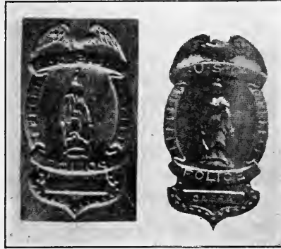
FIG. 79.—Embossed Police-shield before and after trimming.
