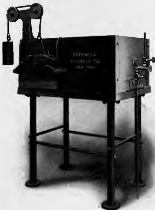
FIG. 163.—End-heating forge furnace.
