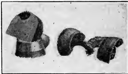
FIG. 303.—A worm-cutter and its chip.
