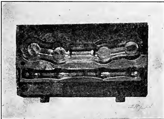
FIG. 15.—Drop-forging die, showing bending-form in front.
