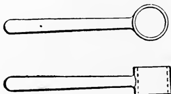
FIG. 28.—Drop-forged shell and handle for ratchet drill.
