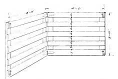
This detachable lambing pen hinged together may be hooked to the wall, other pens may be added as needed, one end being hooked to the corner of last pen and the other to the wall. After lambing panels may then be folded and stored until the next season.
