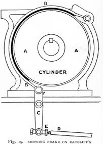
of the rod D. The pressure is regulated in this instance by the screw and regulating nuts, E, at the end of the rod, D.\*
