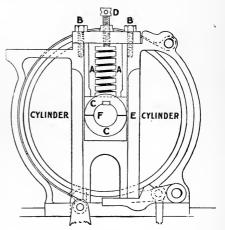
Fig. 15. SHOWING SPRING ARRANGEMENT FOR OBTAINING PRESSURE.
