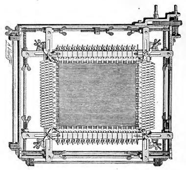
Fig. 23.—FOUGEADOIRE'S IMPROVED REDUCING AND ENLARGING MACHINE.
