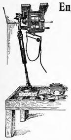
Overhead Litho. Stone Grinding and Polishing Machine. Performs perfect work with
