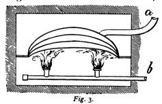
the production of steam for heating the box. *a*, fig. 3, is the pipe passing through the wall into the
