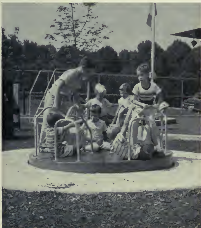
A tanbark area and flush concrete pad surround this merry-go-whirl alongside the Somerton dance and craft terrace.
