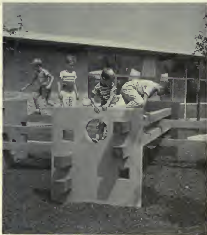
Tanbark area under climbing equipment cushions falls. Many sections of the country use bituminous surfacing instead.
