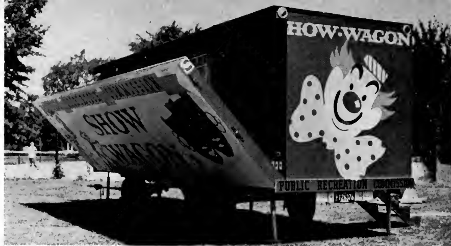
Side lets down by two cables attached to winches mounted on back inside wall.
