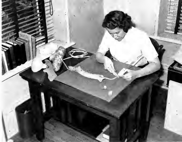
Showing sequence of wiring to be followed after drilling. The felt, cut to shape of base, ready to be glued is shown (left).
