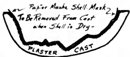
CROSS-SECTION OF PLASTER CAST SHOWING PAPIER MACHE "SHELL" CONFORMING WITH MOLDED FACE. THUS ANY NUMBER OF MASKS MAY BE MADE FROM A SINGLE CAST
