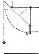
Model 221B swing-up is braced to balcony or wall
