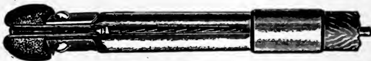
Showing the 3 cleaner pads partly expanded. Each pad is made by stringing 30 brass gauze washers on a holder and compressing to shape shown.
